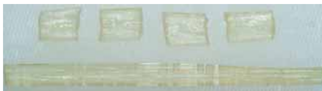
Figure 2. Segments of everStick resin preimpregnated fiber-reinforced composite that are used in the fabrication of a chair-side bridge. Smaller segments are used for shaping the pontic support, and the longer length is used for the wing attachment.
