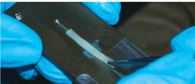
Figure 4. Strips of fiber-reinforced composite are being added to the lower mold.
