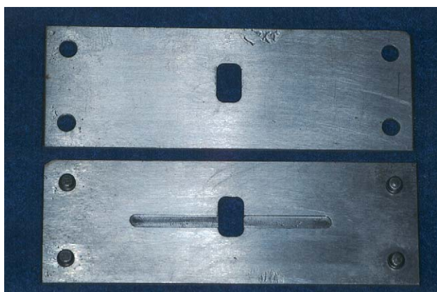
Fig. 3. Custom-made aluminum split mold used in fabrication of FRC frameworks.
